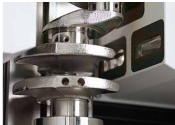
Measuring crank shafts with a HOMMEL-ETAMIC opticlina C1023-75AE
