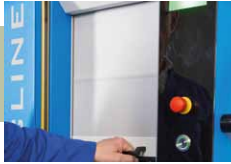
Integrated roller shutter to protect against negative environmental influences (optional)
