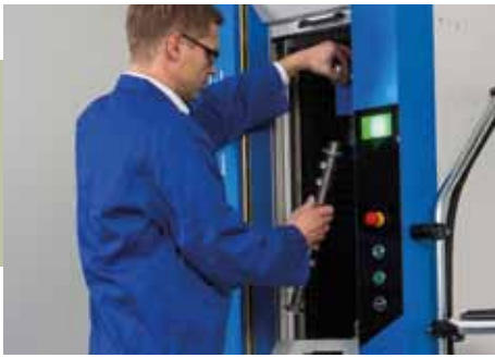
Simple loading of the measuring machine thanks to fast tailstock adjustment
