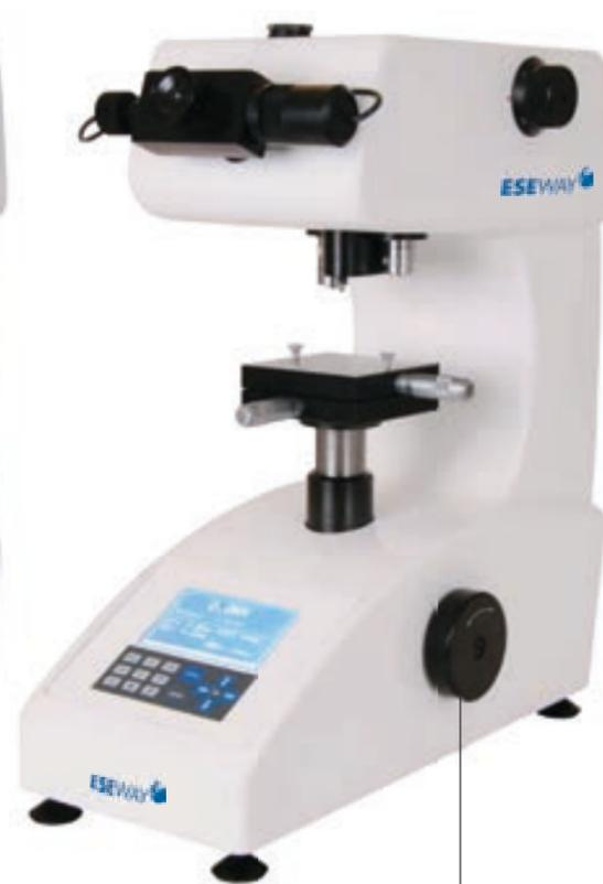
Optional: Electronic handwheel spring loaded, for dynamic Z-Axis movement
