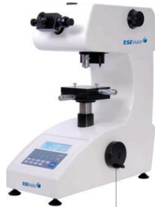
Manual Z-Axis movement, precision adjustment
