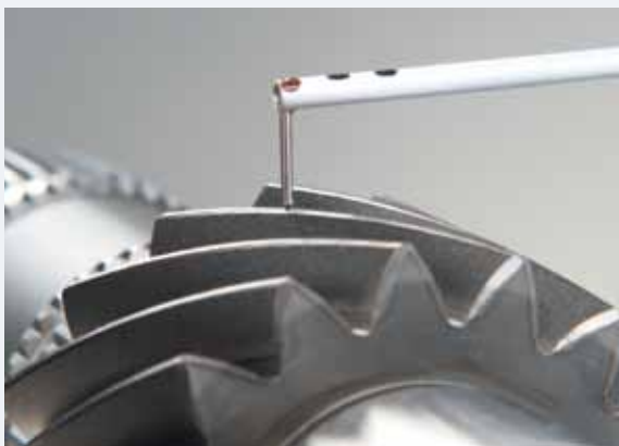
Roughness and contour measurement with one measurement system
