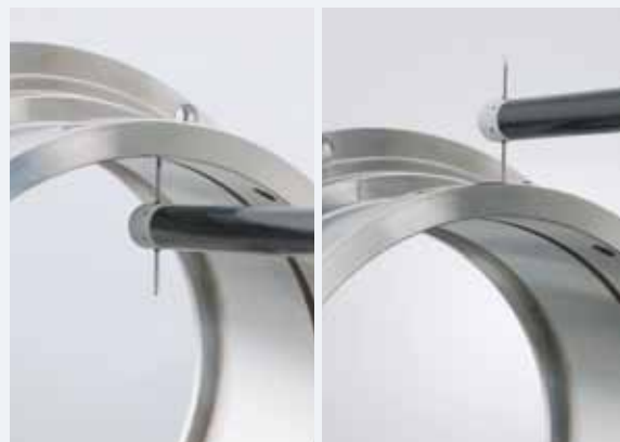
Dual-tip probe arms enable outer/inner measurement.
