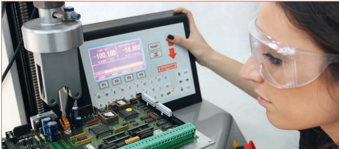
Tensile test on electronic components
