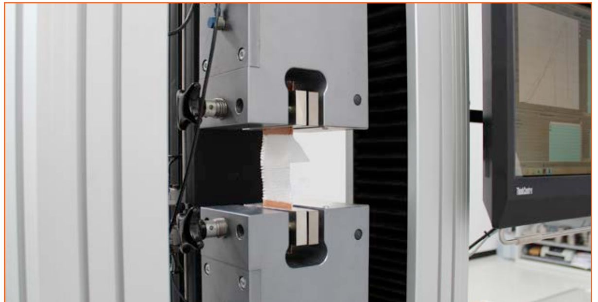
Tensile test on textile, ISO 13934
