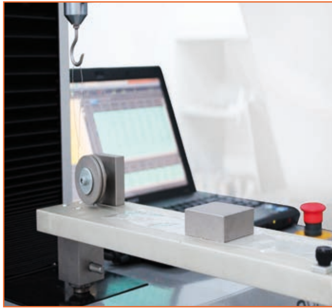
Friction test on plastic film, ISO 8295 - DIN 53375 ASTM D1894 - TAPPI T549
