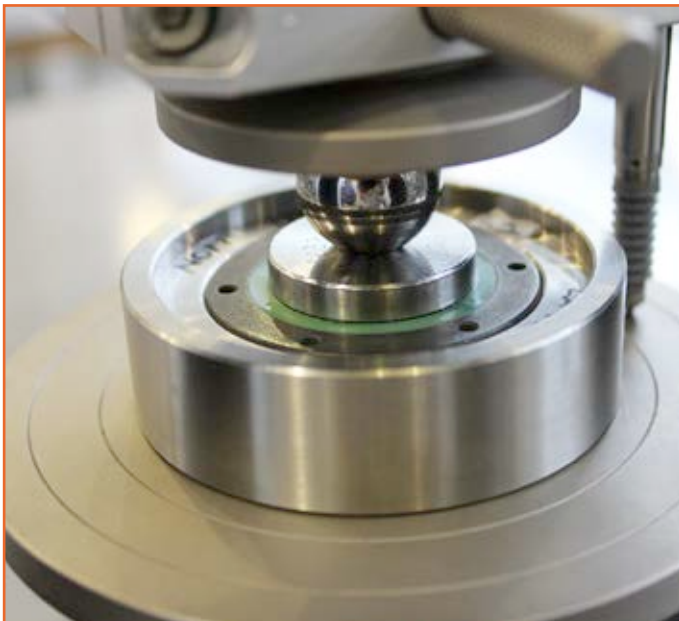
Compression test on rubber O-ring
