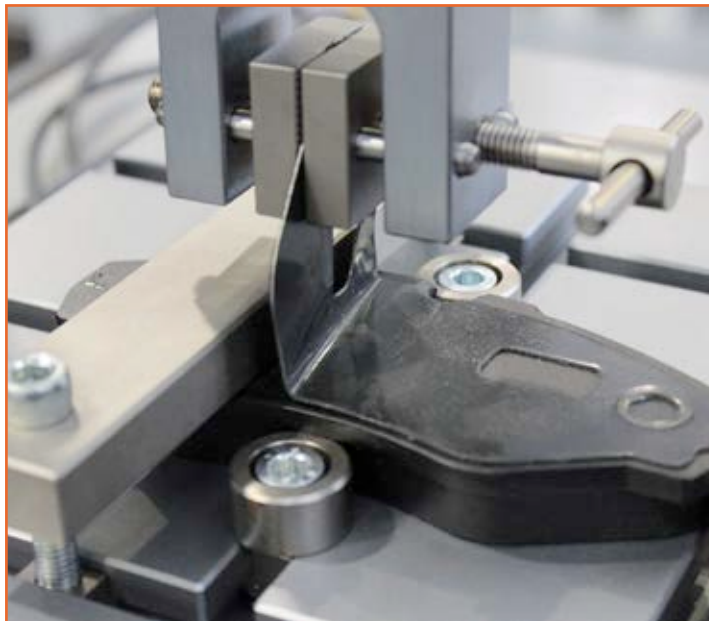
Delamination of brake pad plastic cover
