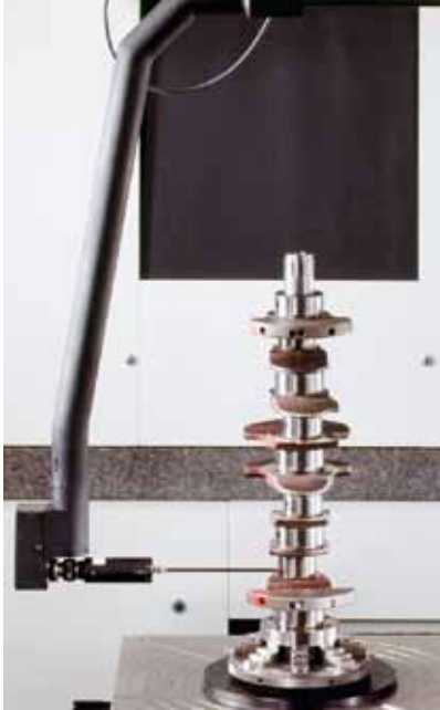
Crank shaft measurement with specific probe arm
