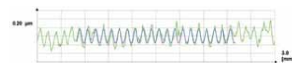
Display of original profile (green) and twist profile (blue)
